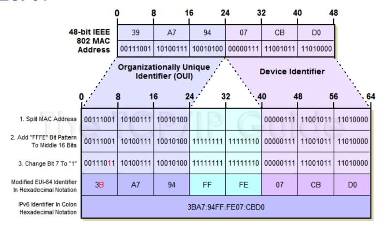
64-Bit IPv6 Modified EUI-64 Interface Identifier
